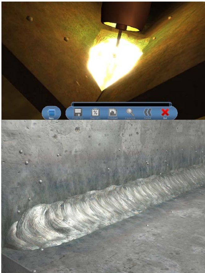
Figure 2: A virtual reality simulation of gas metal arc welding a fillet weld (GMAW). Source: 123 Certification
