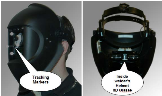
Figure 1: Real Welder Helmet with motion tracking technology Source: 123Certification Inc.
